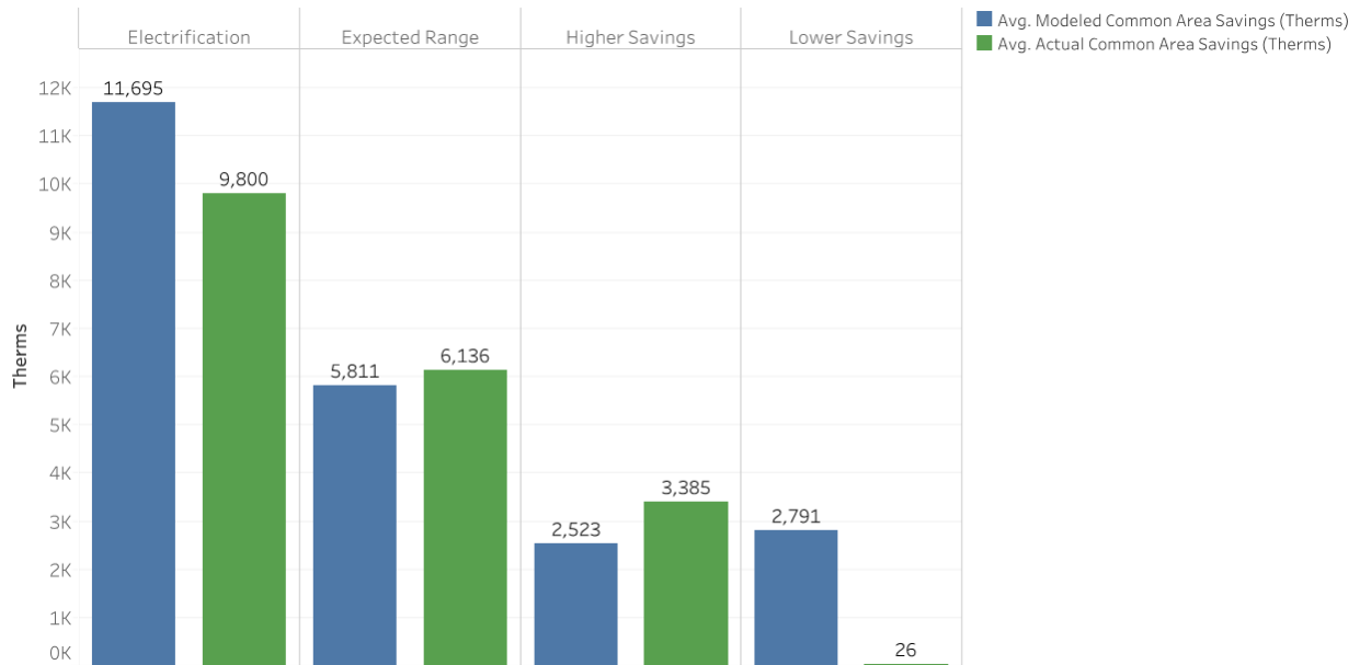
Figure 11 shows the average actual and modeled gas savings for energy conservation measures affecting common areas or central systems. The figure is organized from left to right as follows: electrification (9 projects), savings in expected range (5 projects), savings significantly higher than modeled predictions (10 projects), and savings significantly lower than modeled predictions (19 projects).
